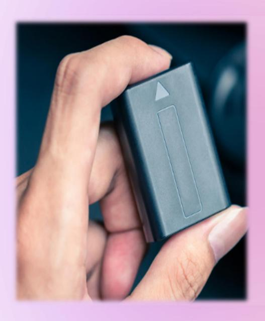
A lithium-ion battery, often known Li-ion battery, rechargeable battery in which lithium ions travel from the negative electrode to the positive electrode via an electrolyte during discharge and then back again during charging.
